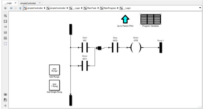
**6** Double-click each new block added to the rung and specify the tags. In Ladder Diagrams, tags (variables) are used for representing all inputs, outputs, and internal memory. The tag can be a variable name or an expression like:
