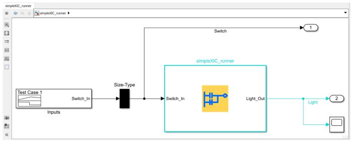
**4** Modify the Signal Builder input to mimic a switch operation as shown.
