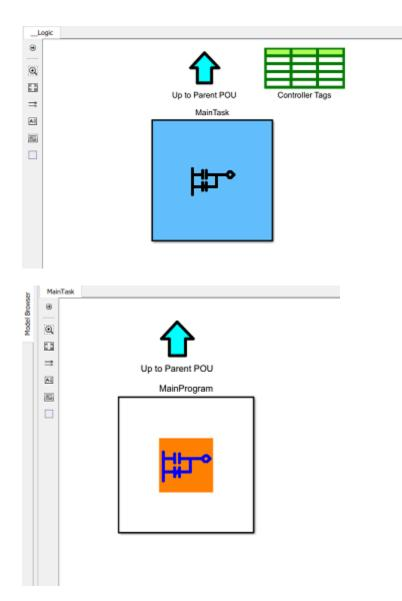
The Main Program contains the Simulink implementation of the simple\_timer.L5X Ladder Diagram. The ladder rung executes from top to bottom and left to right.
