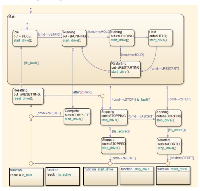
You can map the states and transitions in the chart to the generated code. For instance, the transition from the state Aborting to Aborted appears in the generated code as:
