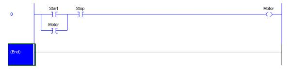
1 Use the plcladderimport function to import the ladder into Simulink.
