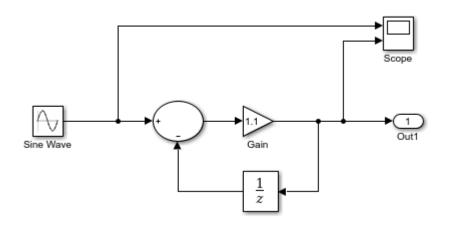
2 Configure the model to use the fixed-step discrete solver. Click the solver link in the lower-right corner. The Solver information pane opens. In the pane, click the View solver settings button to open the Solver pane of the model configuration parameters. Under the Solver selection, set Type to Fixed-step and Solver to discrete (no continuous states).
