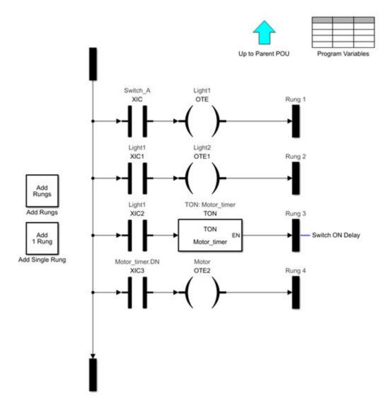
You can use the Signal Builder block to create test inputs for Switch\_A and verify the operation of the imported ladder. You can also generate a PLC Ladder Diagram code or a C code for the top-level subsystem. If you want to edit the imported ladder, the Simulink blocks are in the template Ladder Diagram Library. To open the library, enter:
