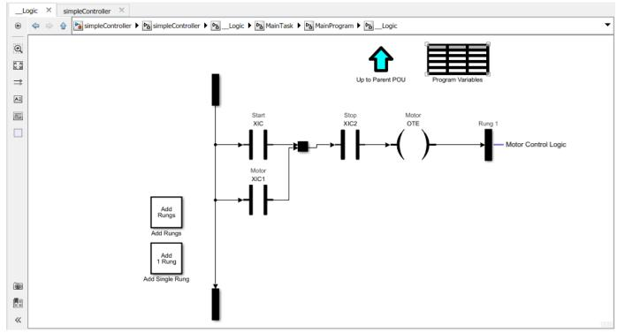
**9** Update the ladder logic model to reflect changes. You have now created a simple ladder model in Simulink.
