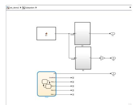
**2** The S1, S2 blocks are identical and contain simple feedback loop. The Stateflow chart contains a simple state machine.
