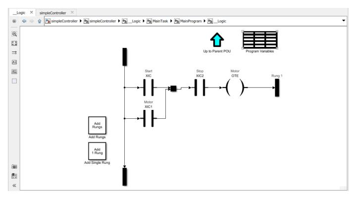
To generate C code for the subsystem, simpleController/simpleController you must first enable 'FastSim' option for the Simulink Ladder Diagram model.
