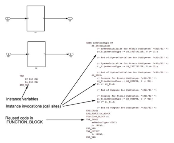
**5** Examine the generated Structured Text code. The code defines FUNCTION\_BLOCK S1 once.
